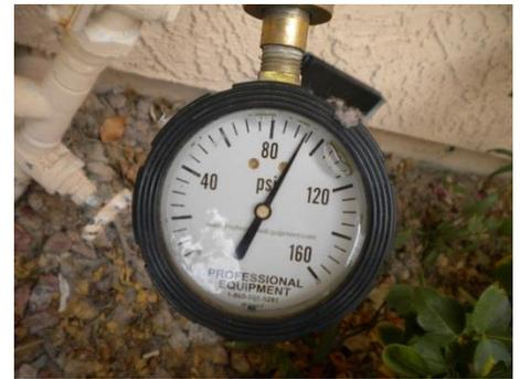
Water is a dynamic fluid with mass. When it is stopped suddenly, the mass of the water increases the force of the water over that of its static pressure. Just like a one pound hammer exerts a much greater force when it comes to a sudden stop at the top of a nail; the force of the water hammer effect may cause pipe joints to break, valves to leak, and over time and repeated occurrences, parts to succumb to the force of the water.
